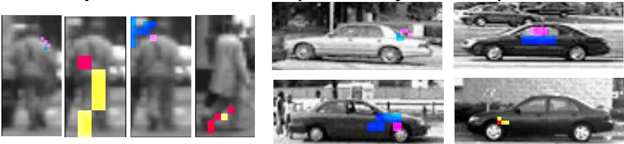
Typical connected-Control-Points selected during Adaboost training
